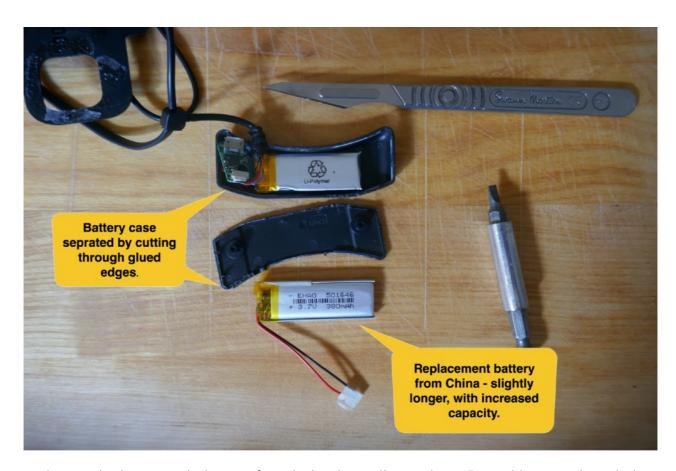
was destroyed, whereas, with the use of a scalpel and a small screwdriver, I was able to cut through the glue linking the two halves and prise them apart, with minimal damage. I purchased two batteries from China for the staggering sum of £10.28, including postage.
